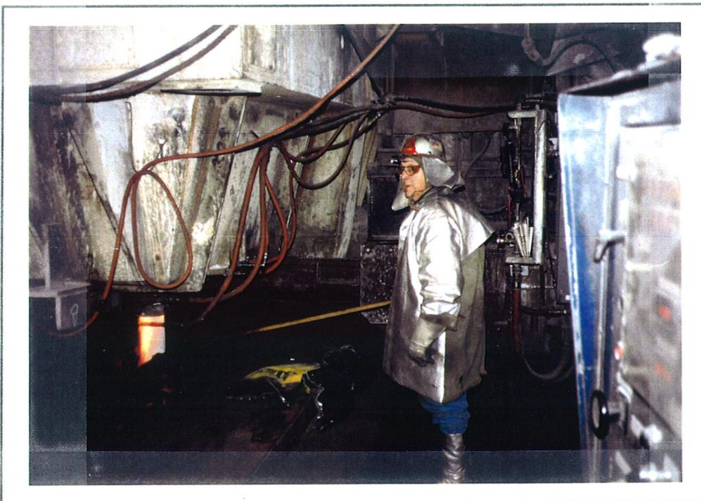
**Figure 5.1(b): Manual Mold Powder Addition**
